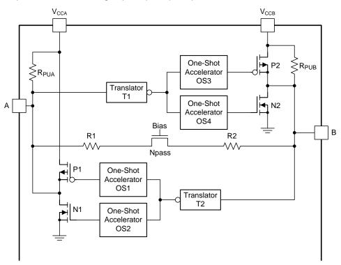
Figure 9. Architecture of a TXS0108E Cell
