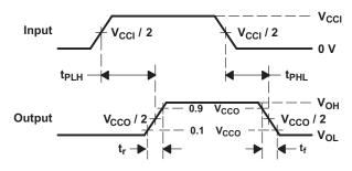
Figure 8. Propagation Delay Times
