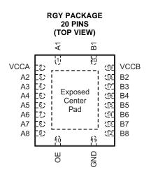
The exposed center pad, if used, must be connected as a secondary ground or left electrically open.
